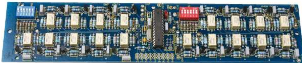
The volume control board, the only component which the Manufacturer wants to keep top secret.
